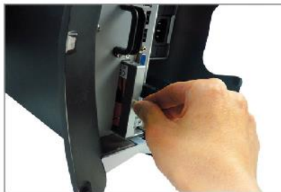
Simple 1-Screw HDD Replacement
